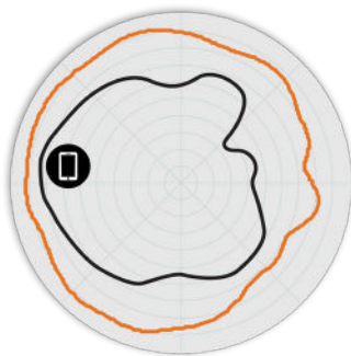
Figure 2. R770 2.4GHz Azimuth Antenna Patterns
