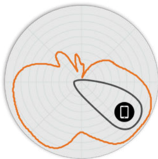
Figure 5. R770 2.4GHz Elevation Antenna Patterns
