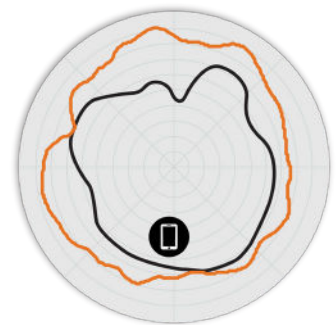
Figure 4. R770 6GHz Azimuth Antenna Patterns
